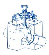
BEL Valves' Check Valve range supports client needs for a flexible approach to solutions where protection against back flow and pressure surges are concerned. The robust design of the Swing Check Valve is typically favoured to overcome these service conditions on large bore applications, whereas the Axial and Piston Check products provide assurance where a more compact design is demanded.
